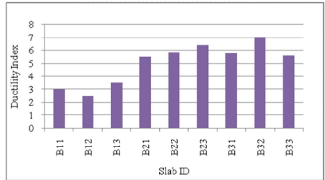
Figure 12. Ductility Index for M30 Slabs
